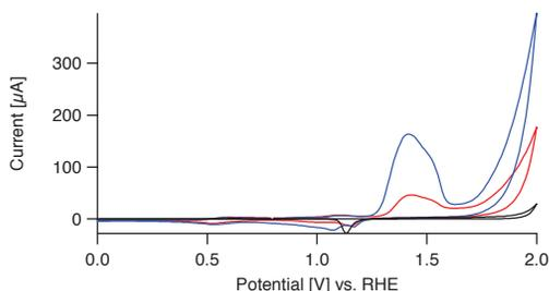
**Figure 2.2:** Voltammogram showing a blank gold working electrode (black) and a gold working electrode in the presence of complex **1** without (red) and with the addition of 6 eq. NaCl (blue). The current of the oxidation peak at ~1.4 V vs. RHE correlates directly with the concentration of Cl<sup>-</sup> ions. Conditions: 0.1 M NaClO<sub>4</sub>, 1.1 mM complex **1**, scan rate 10 mV/s.
