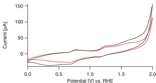
**Figure 2.7:** Comparison of voltammograms of 1.1 mM complex **1** in a 0.1 M NaClO<sub>4</sub> solution at a scan rate of 10 mV/s before (red) and after (black) chronoamperometry (180 s at 1.9 V).
