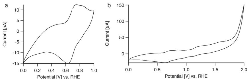
**Figure 2.4:** Results of a CV measurement of 1.1 mM complex **1** using a PG working electrode in a 0.1 M NaClO<sub>4</sub> solution measured at 10 mV/s with a starting potential of 0.7 V vs. RHE with a scan range of (a) 0.0 to 1.0 V vs. RHE and (b) 0.0 to 2.0 V vs. RHE.
