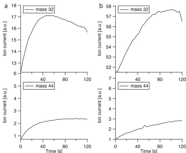
**Figure 2.5:**  $m/z$  traces of O<sub>2</sub> (top) and CO<sub>2</sub> (bottom) recorded during chronoamperometry measurements in a 0.1 M NaClO<sub>4</sub> solution with 1.1 mM of (a) complex **1** at 1.9 V vs. RHE and (b) complex **2** at 2.0 V vs. RHE.
