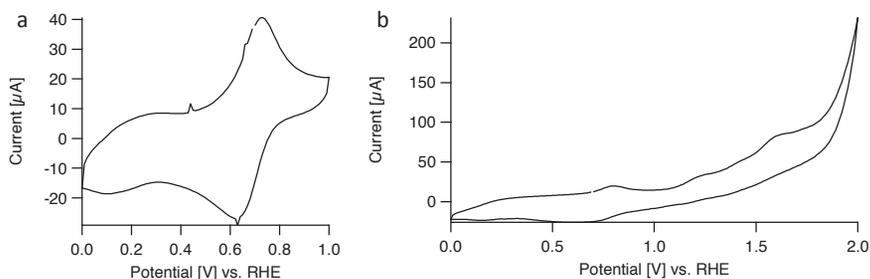
**Figure 2.8:** Results of a CV measurement of 1.1 mM complex **2** using a PG working electrode in a 0.1 M NaClO<sub>4</sub> solution measured at 10 mV/s with a starting potential of 0.7 V vs. RHE with a scan range of (a) 0.0 to 1.0 V vs. RHE and (b) 0.0 to 2.0 V vs. RHE.
