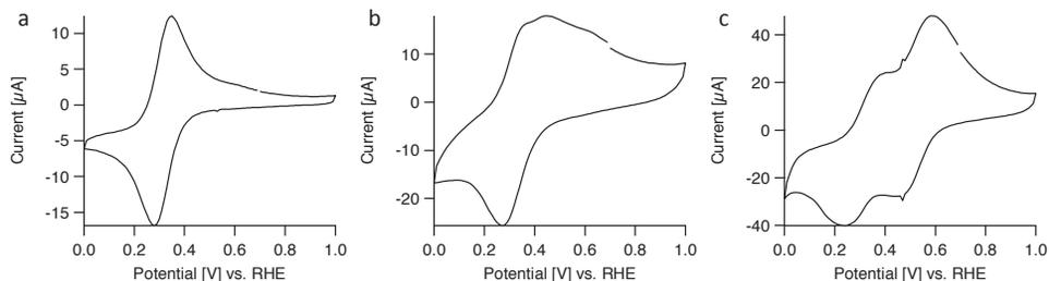
**Figure 2.10:** Results of CV experiments, showing the Fe<sup>II/III</sup> redox couples of complex **1** (a), complex **3** (b) and complex **2** (c), each in a 0.1 M phosphate buffer solution (pH 7.5). All three CVs were recorded at 10 mV/s between 0.0 and 1.0 V vs. RHE with a starting potential of 0.7 V vs. RHE.
