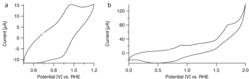
**Figure 2.9:** Results of a CV measurement of complex 1.1 mM **3** using a PG working electrode in a 0.1 M NaClO<sub>4</sub> solution measured at 10 mV/s with a starting potential of 0.7 V vs. RHE with a scan range of (a) 0.0 to 1.0 V vs. RHE and (b) 0.0 to 2.0 V vs. RHE.
