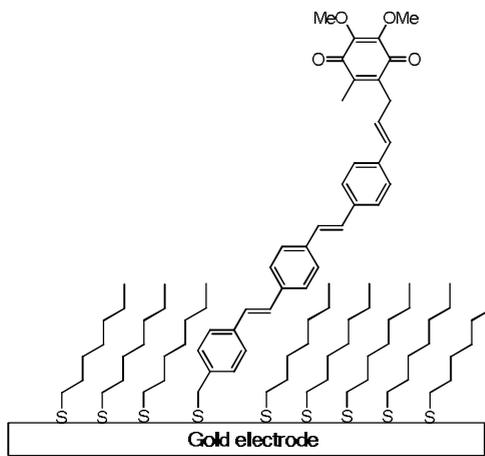
**Figure 1** Visualization of the surface of a gold electrode modified with a Q-wire ( $U_3$ ) and heptanethiol
